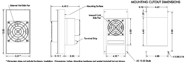
\* Dimension does not include hardware, insulation. Dimensions: Inches, Mounting hardware and gasket included but not shown. † On all models of AHP-300X, these dimensions are greater by 0.25 inch.
